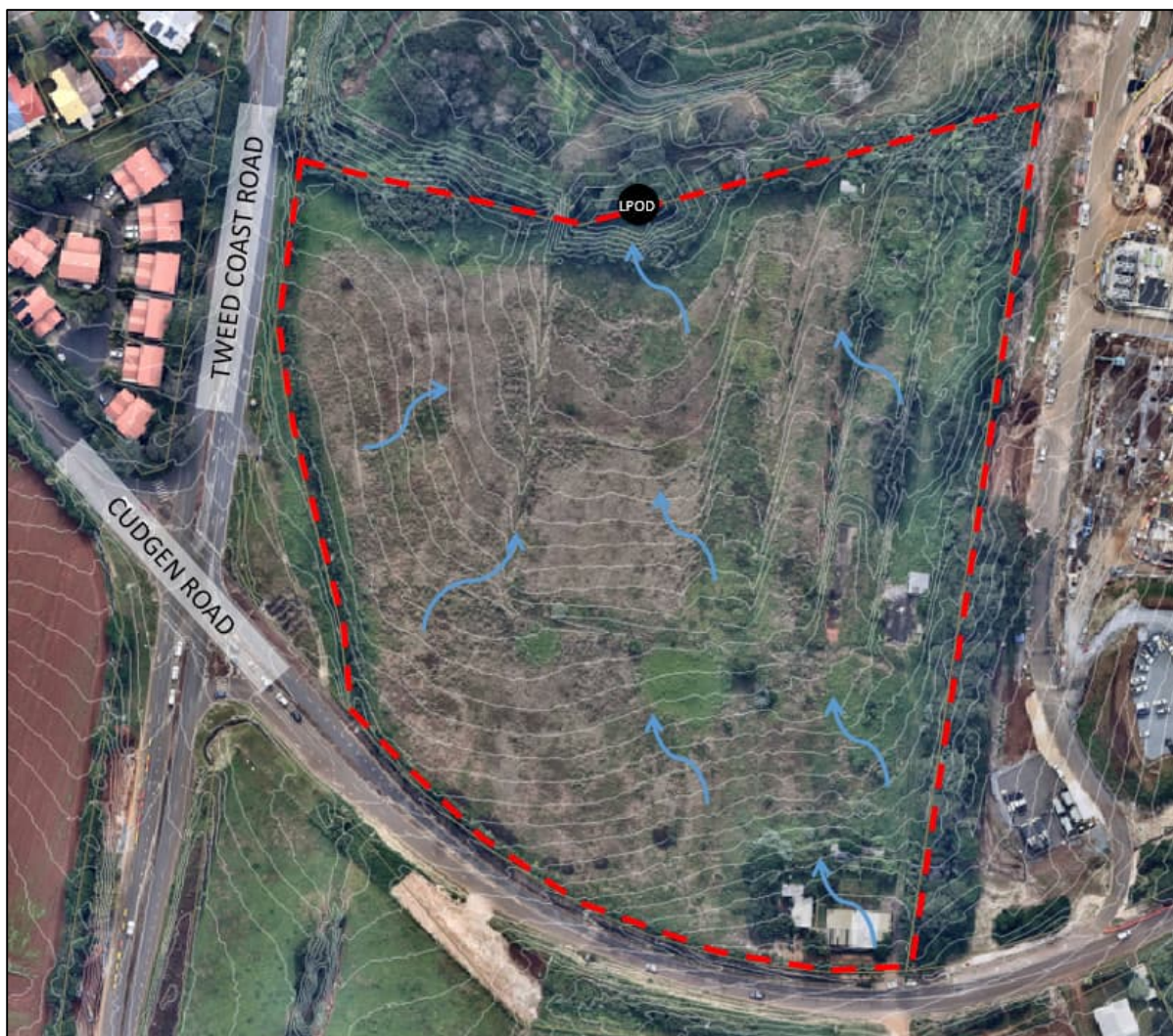
Figure 3: Existing Stormwater Conveyance
